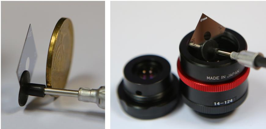
Fig. 39: The 130  $\mu\text{m}$  mask (left) and the 'Kowa LM16JCM-V' two-part 16mm lens.
