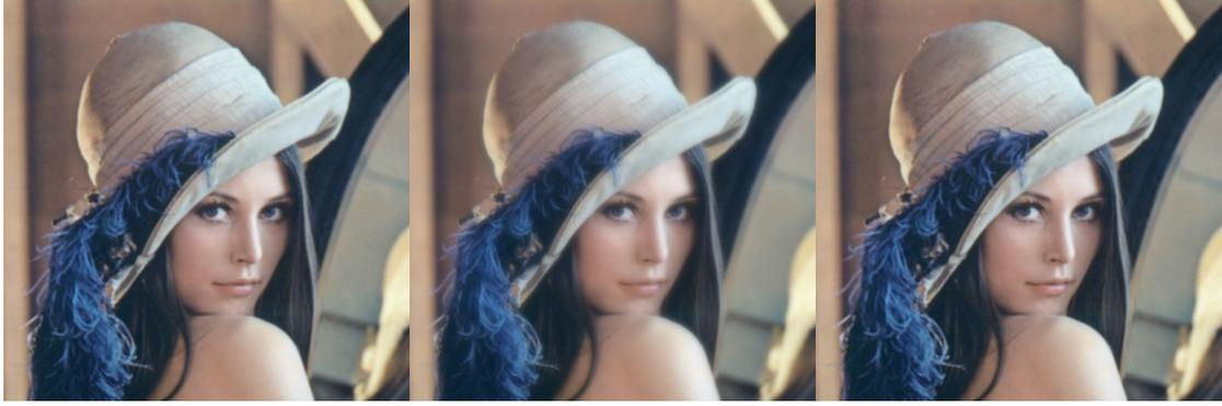
*Fig. 30: Imaging with DLIM lens (left – PSNR 26.3dB), with uncorrected lens (center – PSNR 23.7dB) and with a phase mask (right – PSNR 25.4dB).*
