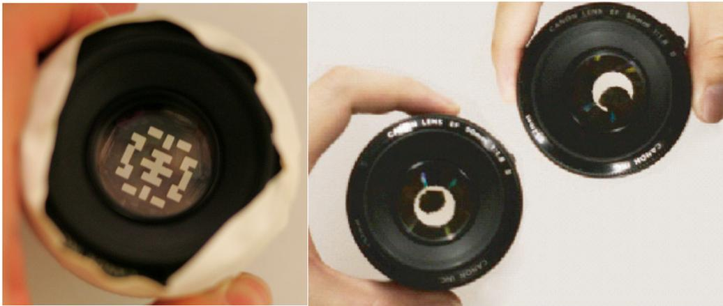
*Fig. 14: Amplitude masks example: left - Levin et al. [31]; right - Zhou et al. [45]*
